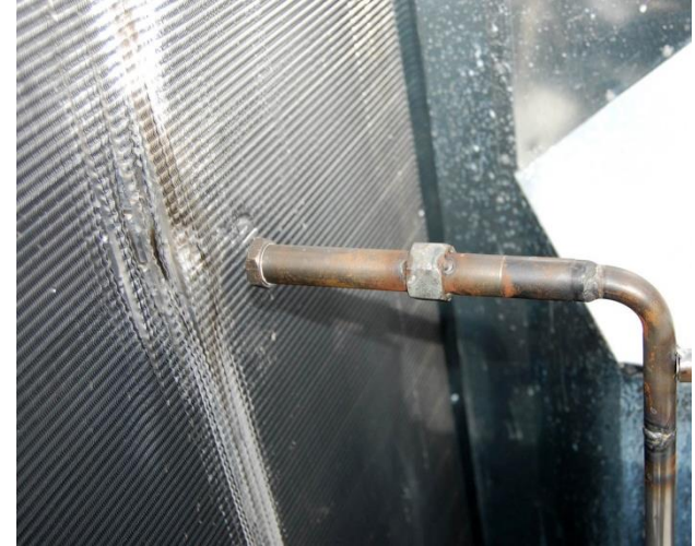
Damage of lamellas during test P4
