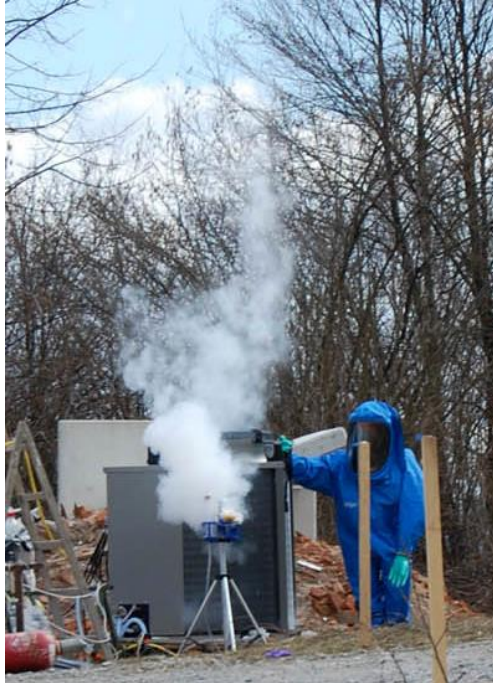
Cloud of ammonia during test P4
